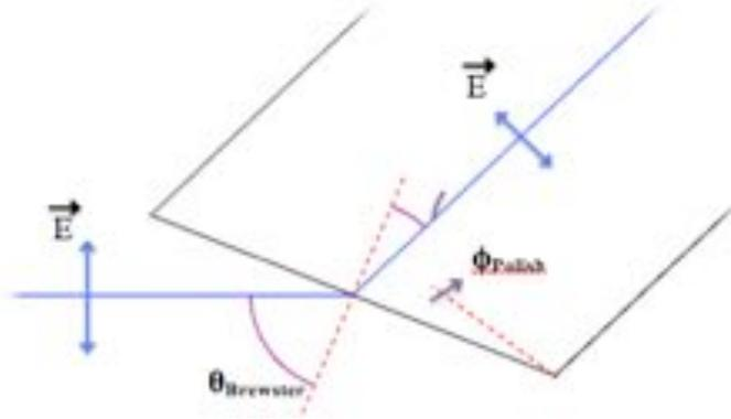
Figure 2: Diagram showing the input beam polarization for maximum transmission. Additionally the relevant angles are shown
