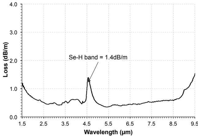
Figure 7. Loss spectrum for the 200/250  $\mu\text{m}$  As-Se fiber.
