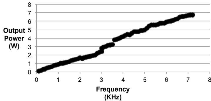
Figure 8. Output power transmission versus modulation frequency for As-Se fiber with CO<sub>2</sub> laser at 9.3  $\mu\text{m}$ .
