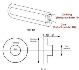
The core and cladding have different refractive indices. The refractive index of the core,  $n_1$ , is always greater than the index of the cladding,  $n_2$ . The core transmits an optical signal while the cladding guides the light within the core. Since light is guided through the fiber it is sometimes called an optical wave guide
